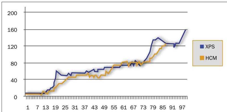
**Figure 1.** Instantaneous RSS ( $\mu$ strain) recorded over time (seconds) by the strain gauge attached to the apical third of the mesial root during instrumentation of MB and ML canals by XPS and HCM files respectively.
