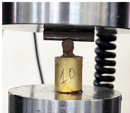
Figure 1 Compression test set-up.
