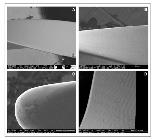
Figure 1 Surface of new files: BRO (A), BR1 (B), BR2 (C) and BR3 (D).
