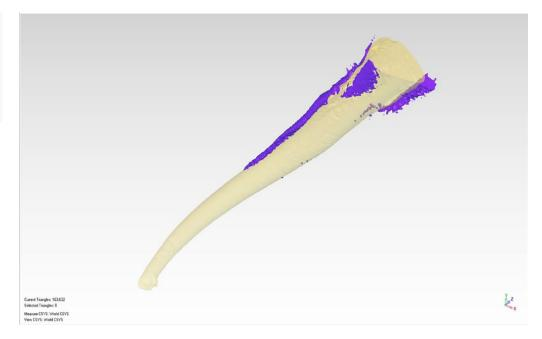
done, each acquisition was reconstructed with the software NRecon (©2012 Bruker) using standardized parameters for the whole study: 15% beam hardening; artifact correction between 4 and 8, depending on the specimen's artifact; smoothing between 3 and 5, depending on the specimen's radiodensity: Output histogram as well was standardized on the HU scale (min: 0; max: 0.064) (figure 1).
